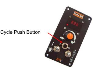
The Cycle Push Button is used to enter the programmable parameters menu that allows the operator to change their values and settings and so define how the automatic cycle will function. The Cycle Push Button is located between and above the Run/Stop switch and the Forward/Neutral/Reverse switch of the GSP control.
